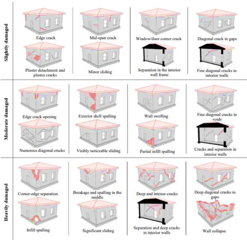
Figure 4. Examples of masonry structures classified as light, moderate or heavy damaged
