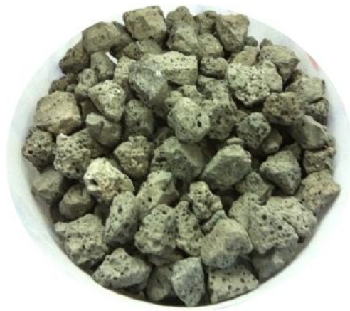
Figure 10 Steel slag aggregates
