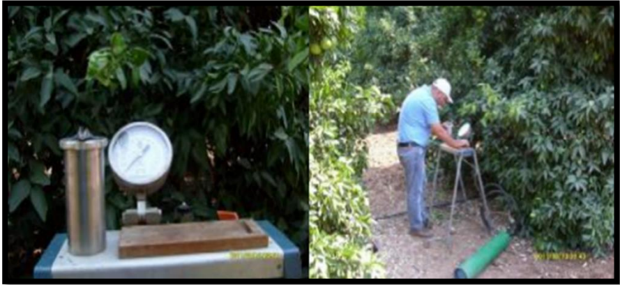
Figure 1. The LWP measurements and the LWP equipment.
