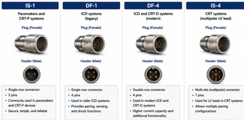
Figure 4: Connector standards used in contemporary cardiac implantable electronic devices
