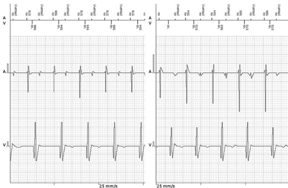
Picture 3:Far-field R-wave (FFRW) oversensing
