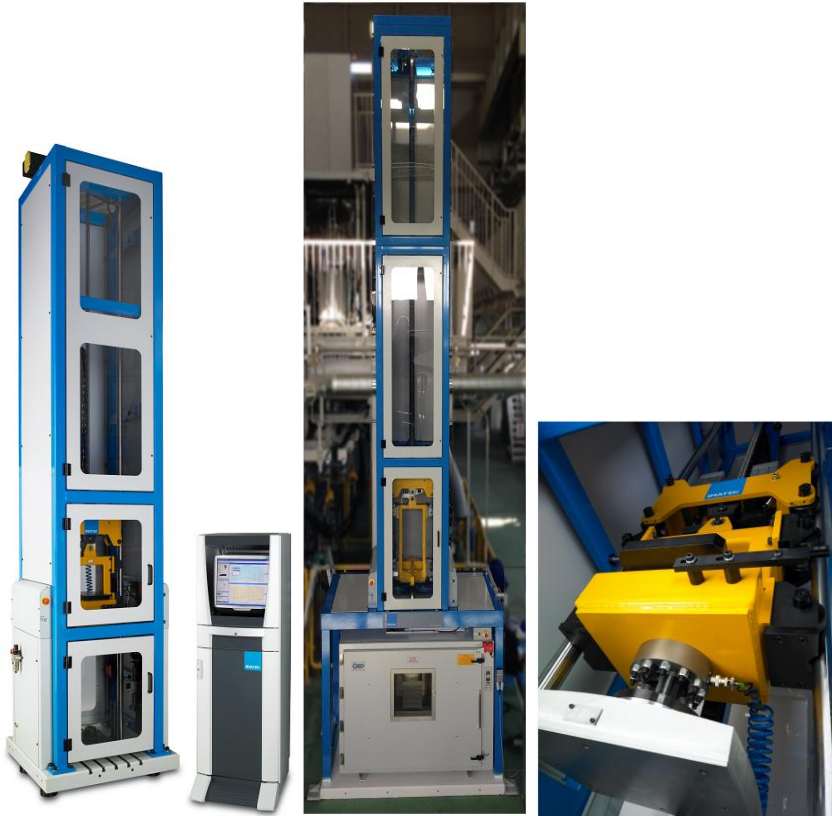
Figure 4 Imatek IM100 Series drop weight impact testing machine.
