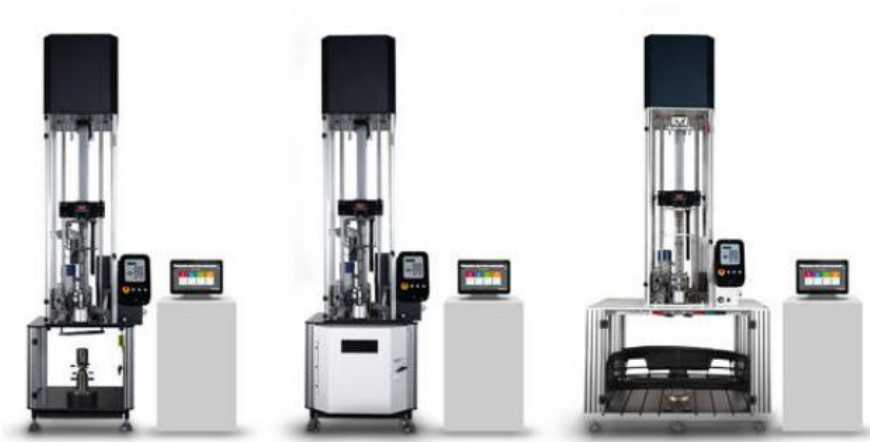
Figure 2 Instron 9400 Series drop weight impact testing machine
