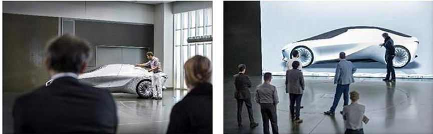
Figure 7 . Design Review of the BMW Vision 100 show car using a physical 1:1 model (Left) and a VR-based model (Right)
