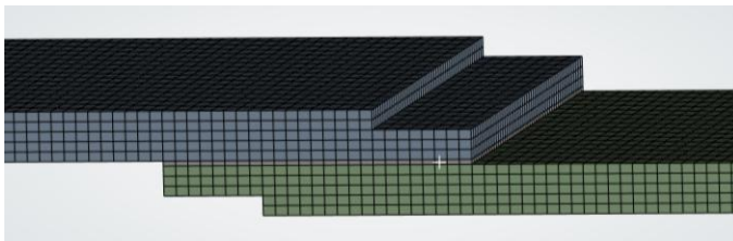
Figure 2. Representative FE mesh for the adhesively bonded joint model.
