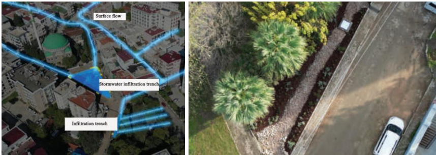
Figure 13 Infiltration trench of the Buca Atatürk Neighborhood Sponge Park and surface runoff to be collected within the project area
