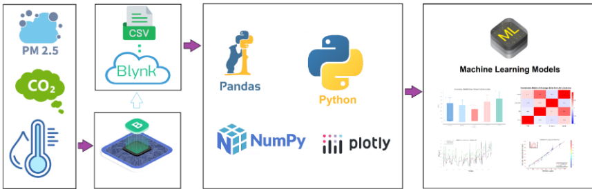
Figure 2. Sensor Data Collection and Calibration Process of IoT-Based Air Quality Monitoring System
