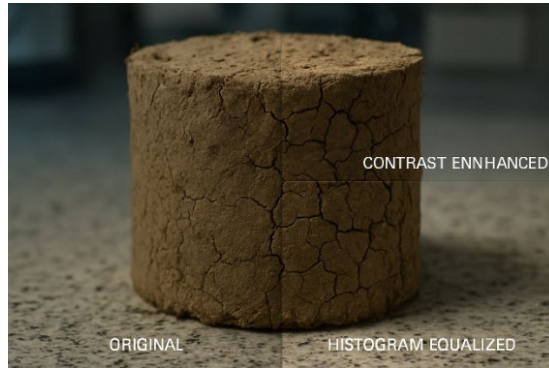
Figure 3: Example of filtering and contrast enhancement in image pre-processing stage
