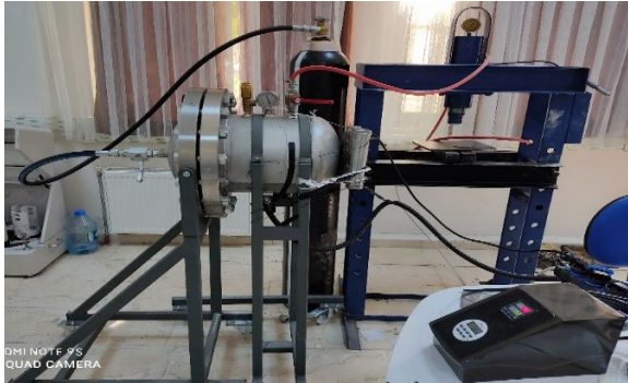
Figure 5. Experimental setup used for supercritical drying
