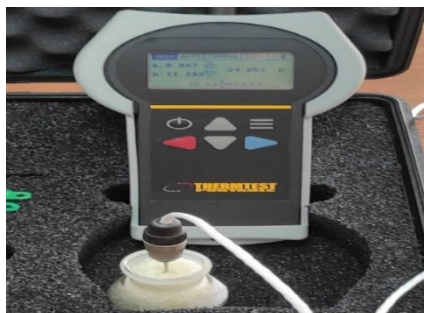
Figure 7. Determination of thermal conductivity of the produced aerogels
