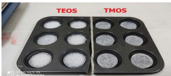
Figure 6. Dried circular aerogels synthesized from TEOS and TMOS
