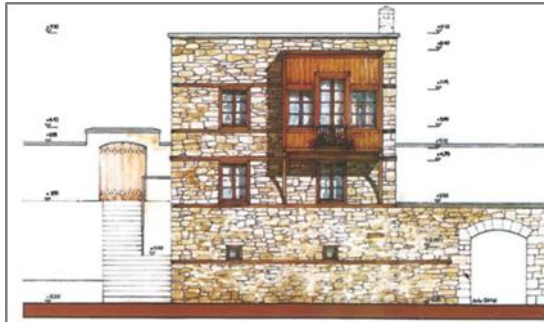
Figure 6. Example of the Connection of Stone Wall and Wooden Beams: Şefik Gül Cultural House West Façade
