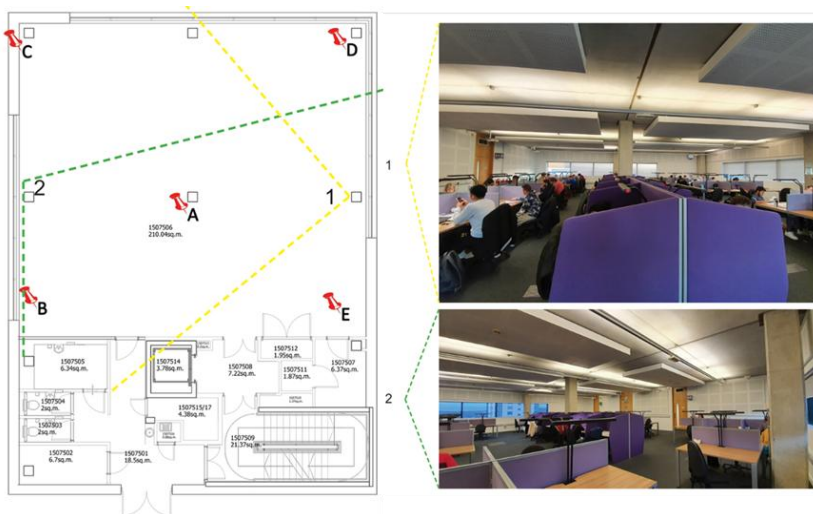
Figure 3. Floor plan of the 5th Floor Silent Room showing measurement points (A-E).
