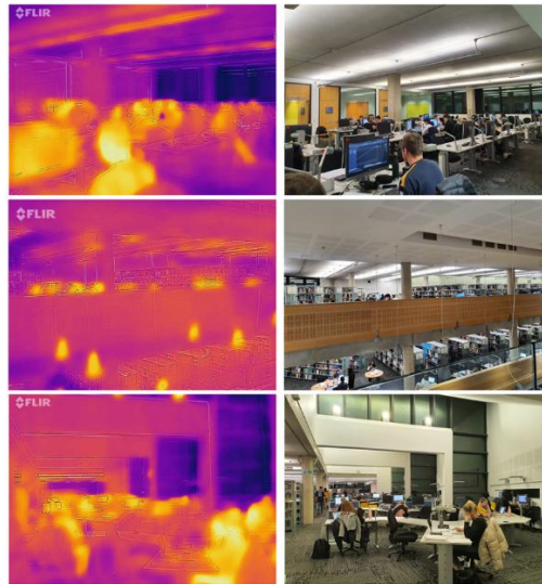
Figure 5. Thermal imaging (FLIR) of the 4th Floor General Study Area showing surface temperature distribution.
