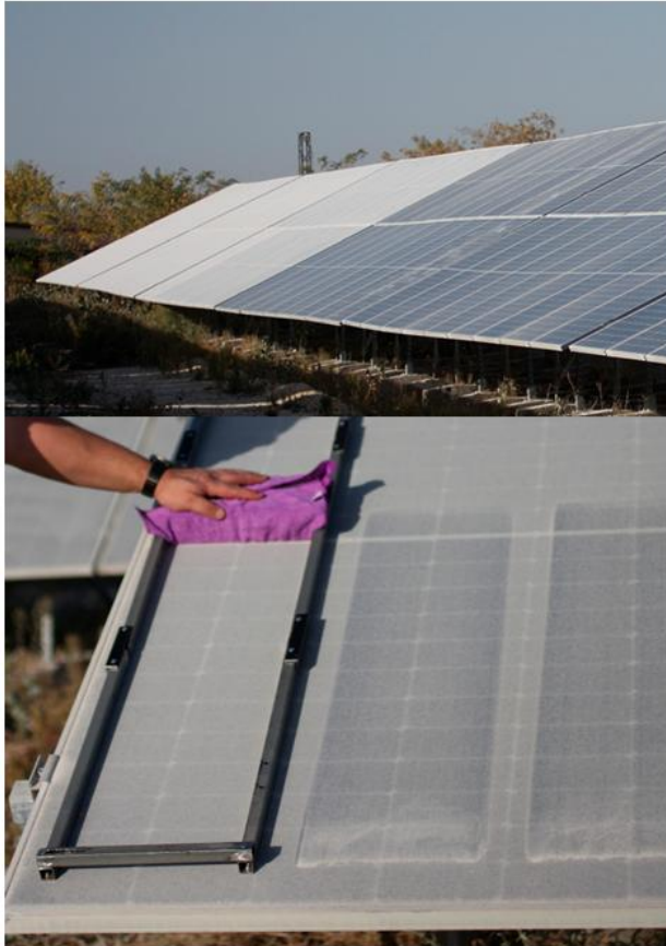
Figure 7. Visual characteristic of a PV panel contaminated with limestone dust and the establishment of resistance to the accumulated dust layer.
