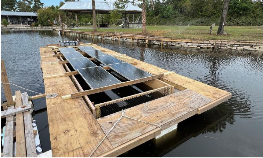
Figure 2. FIPRS test platform constructed of wood and flexible siding/flooring material, with floating collar, and converted to DC power with solar system.
