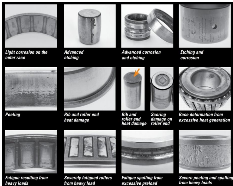
Figure 2: Some Example of Bearing Damages
