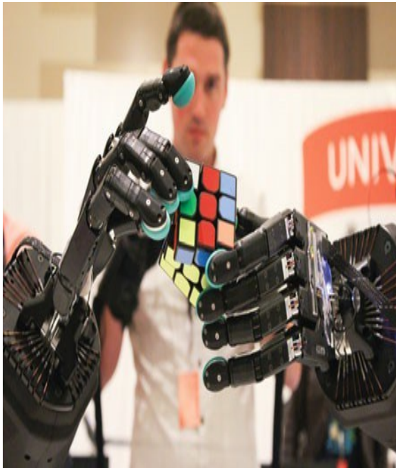
Figure 1.19 showcases the fully actuated Shadow Dexterous Hand by Shadow Robot Company, integrated with BioTacs sensors from SynTouch. This system enables precise manipulation with direct contact force and direction measurement for each fingertip. Image courtesy of Shadow Robot Company, Qc 2022, used with permission.
