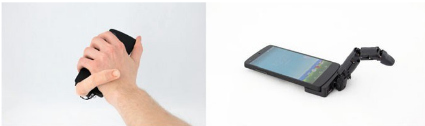
Figure 1.5 showcases the MobiLimb project, a novel exploration by Marc Teyssier that introduces a device capable of "touching back." This work delves into the boundaries between human and robotic interaction, questioning what is socially acceptable in this emerging field. The image is credited to Marc Teyssier, Qc 2022, and is used with permission (Teyssier et al., 2018).
