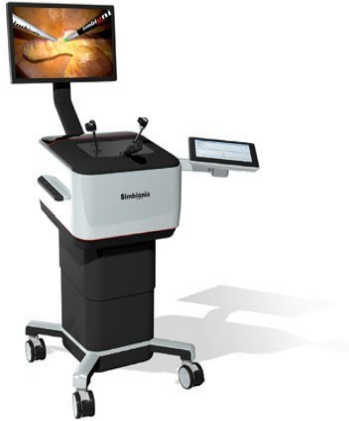
Figure 1.13 Depicts the LAP Mentor III laparoscopic simulator, designed to replicate abdominal interventions. Image courtesy of Symbionix USA, Cleveland, OH, USA, used with permission.
