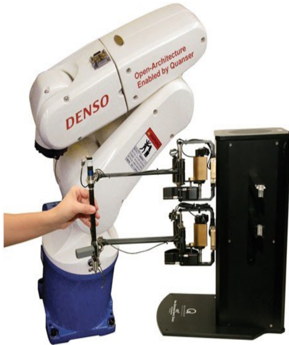
Figure 1.10 illustrates versatile teleoperation using Quanser's HD2 haptic interface, which provides 7 degrees of freedom (DoF) of haptic feedback, paired with the Denso Open Architecture robot offering 6 DoF. Image courtesy of Quanser, Markham, Ontario, Canada, used with permission.
