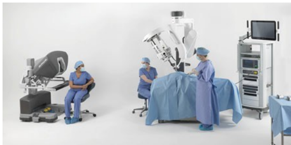
Figure 1.12 depicts the Da Vinci SP surgical system designed for single-port access. Image courtesy of Intuitive Surgical Operations, Inc., Qc 2022, used with permission.
