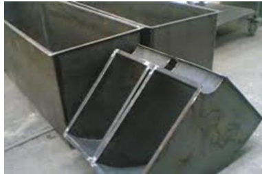
Figure 2. Ventilation duct constructed from black steel sheet (Alafcohvac 2025).
