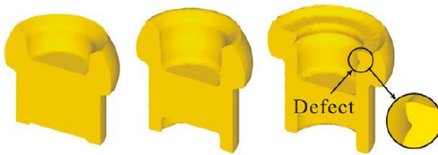
Figure 4: The buckling defect in an axisymmetric part manufactured with the cold forging method. (W.L. Chan,2009)
