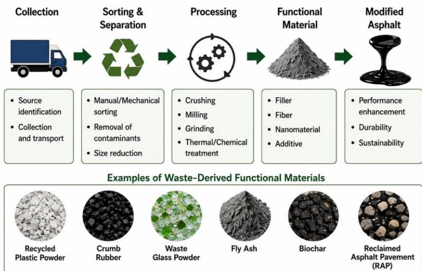
Figure 4.3. Processing route that converts collected waste streams, through sorting, cleaning and treatment, into functional pavement materials and modified asphalt.
