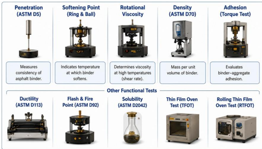
Figure 5.3. Physical and empirical binder tests, penetration, softening point, viscosity, density and adhesion, alongside the ageing tests that complement fundamental rheology.
