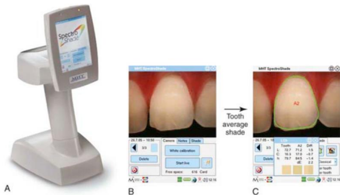
Figure 8. A) SpektroShade B-C) Numerical comparison of color parameters of natural tooth and selected color (Abdulsamee & Nagi, 2020)
