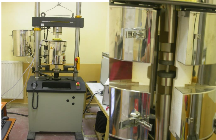
a) Creep testing machine
