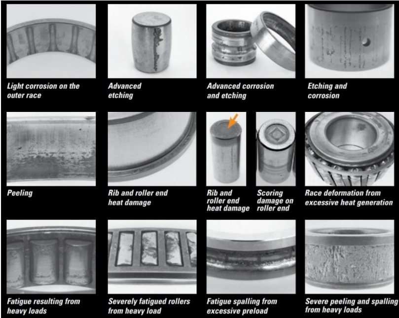
Figure 2: Some Example of Bearing Damages
