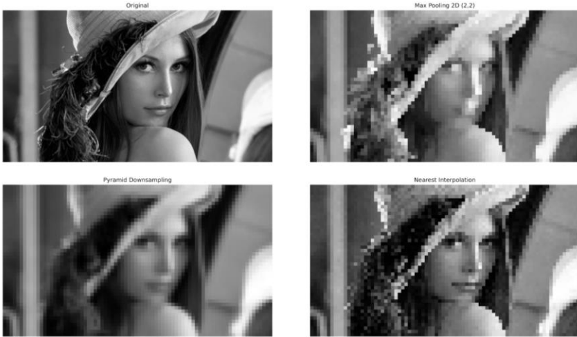
Figure 9: Stage-4 resolution reduction at 80x45 pixel size.
