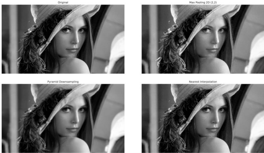
Figure 7: Stage-2 resolution reduction at 320x180 pixel size.
